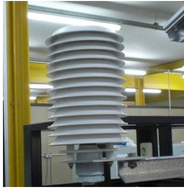
Screen housing temperature and humidity sensors
