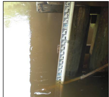
Gauge board and stilling well
