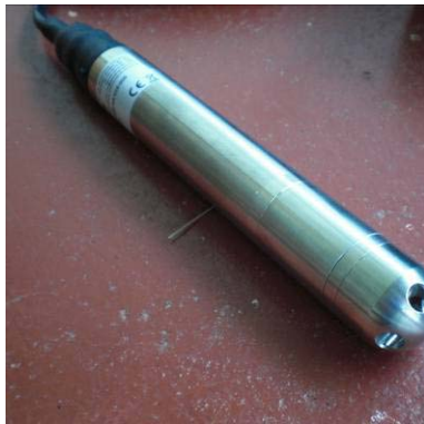
Water level pressure sensor
