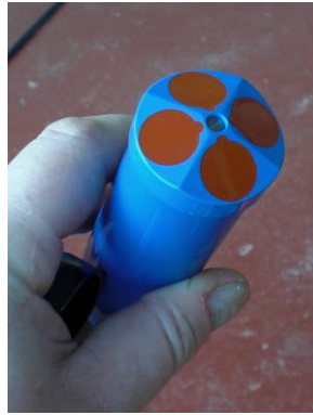
ADCP sonic transmitter / receiver
