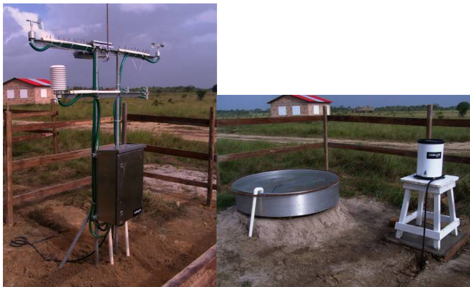
Figure 3 Bina Hill Institute Automatic Weather Station (left) with tipping bucket rain gauge and evaporation pan (right).
