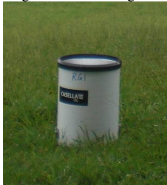
Tipping bucket raingauge being tested in the field
