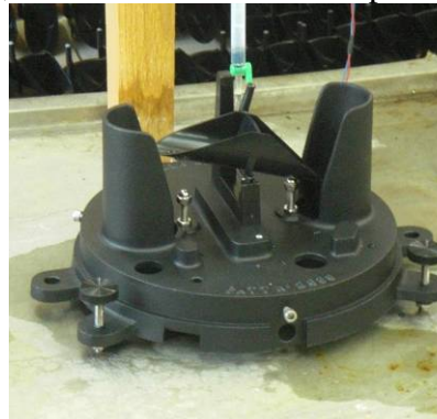
Tipping mechanism inside tipping bucket raingauge
