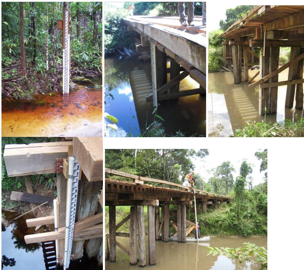
Figure 5 Stage (river level) gauges at Tiger Creek, 8-mile Creek, Big Turu Creek, Blackwater Creek, and Kuipari Creek (top left to bottom right). Water quality probes are also installed at Tiger Creek and Blackwater creeks.
