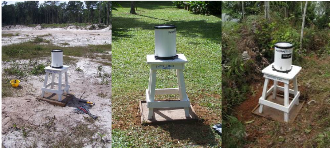
Figure 4 Tipping Bucket Raingauges at Tiger Woods Inc (left), Canopy Walkway (centre) and Turtle Mountain (right)
