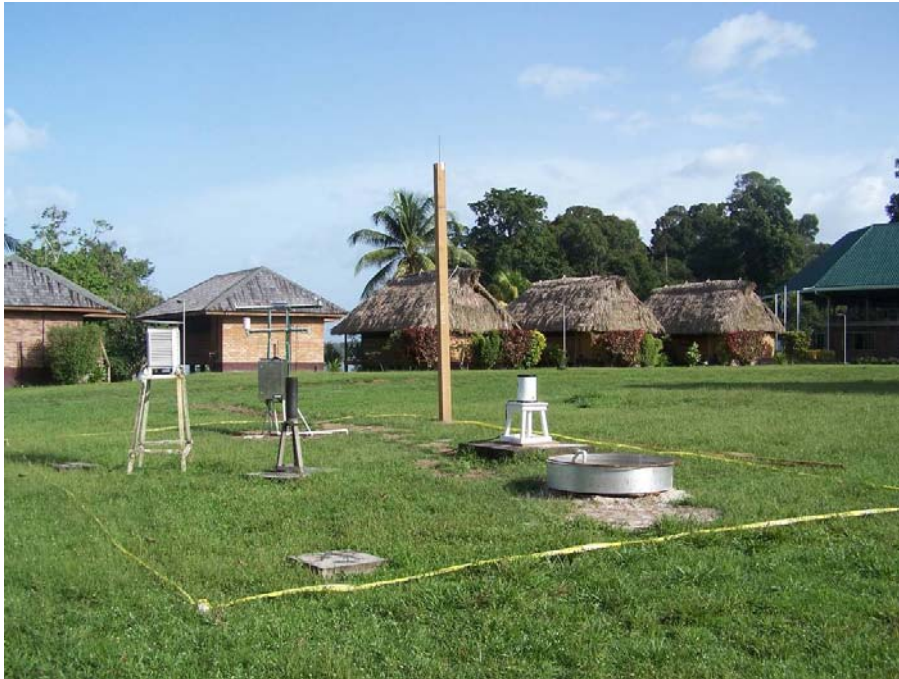
Figure 2 Iwokrama Field Station Automatic Weather Station (centre back) with tipping bucket rain gauge and evaporation pan (right), older manual rain gauge (centre front) and older casing for manual humidity and temperature sensors.
